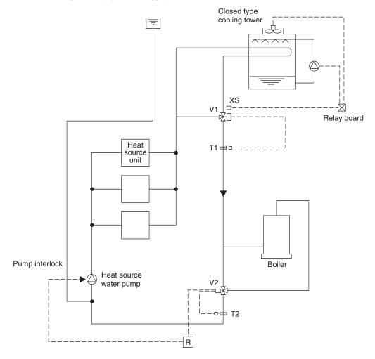
In the summer, as the circulation water temperature rises exceeding the set temperature of T1, the bypass port of V1 will close to lower the circulation water temperature. In the winter, if the circulation water temperature drops below 25°C, V2 will conduct water temperature control to keep the circulation water temperature constant.
