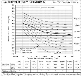
. When Night Mode is set, the A/C system's capacity is limited. The system could return to normal operation from Night Mode automatically in the case that the operation condition is severe.
