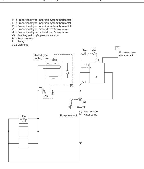
=In the summer, as the circulation water temperature rises exceeding the set temperature of T1, the bypass port of V1 will open to lower the circulation water temperature. In the winter, if the circulation water temperature stays below 25°C, V2 will open/close by the command of T2 to keep the circulation water temperature constant.
