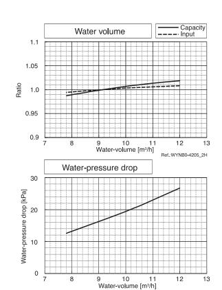
CITY MULTI™ could have varied capacity at different designing temperature. Using the nominal cooling/heating capacity value and the ratio below, the capacity can be observed at various temperature.
