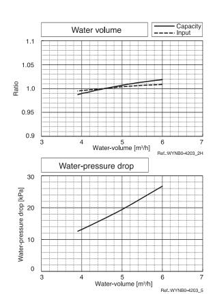
CITY MULTI™ could have varied capacity at different designing temperature. Using the nominal cooling/heating capacity value and the ratio below, the capacity can be observed at various temperature.
